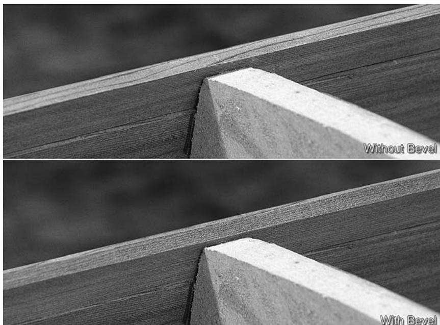
**Figure 13-23.** Usually you only need to bevel a new strip to match the angle of a strip already installed. However, when you have a sharp angle between subsequent strips, you will get a stronger joint by beveling both adjacent strips. It is easier to bevel the first strip before it is installed, but you could use a rabbet plane to bevel after installation.
