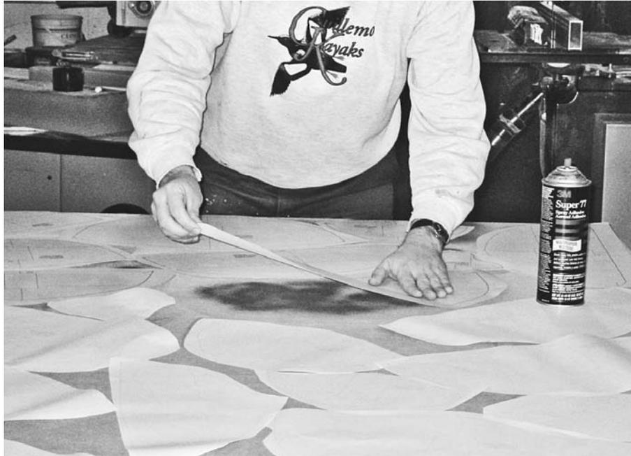
**Figure 4-3.** Instead of transferring lines from the drawing to your form material, cut out full-size drawings, glue them to the form material with spray adhesive, and cut out around the lines. This way all the reference lines are included on the forms.
