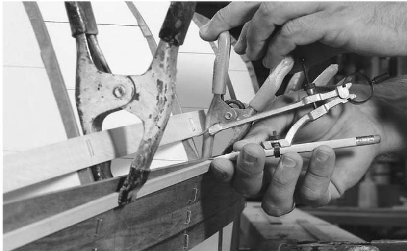
**Figure 12-15.** Staple a strip on the mark you just made and check that it is fair. Then use your compass again to adjust the location of another strip clamped to the installed strips. When this strip is smooth and fair, mark a pencil line along the top edge of this strip. This indicates where you will trim the excess off the existing strips. A Japanese pull saw does a good job cutting off the excess. Cut a little above the line.
