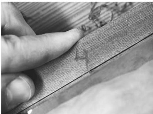
**Figure 6-7.** Keep planing until the gap between the strip and the plane just about disappears. Place the strip back on the forms, making sure to align the number with the appropriate form. Check the gap again. Plane some more, matching the new gap as you start, and plane until the gap disappears. Double-check your fit.
