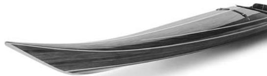
**Figure 10-15.** You can get results almost as good as spraying by careful brushing followed by rubbing out and polishing the result. This Night Heron was sanded with 600- through 2,000-grit sandpaper and then buffed with polish.
