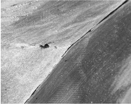
**Figure 10-5.** It is extremely easy to sand through sharp edges and feature lines. Avoid touching these corners with a power sander. You would likely go through the material before you can blink. Instead, keep the pad of the sander flat on the large surfaces, leaving the corners shiny until you are done with all the power sanding, then hand sand with fine sandpaper to lightly remove the gloss.
