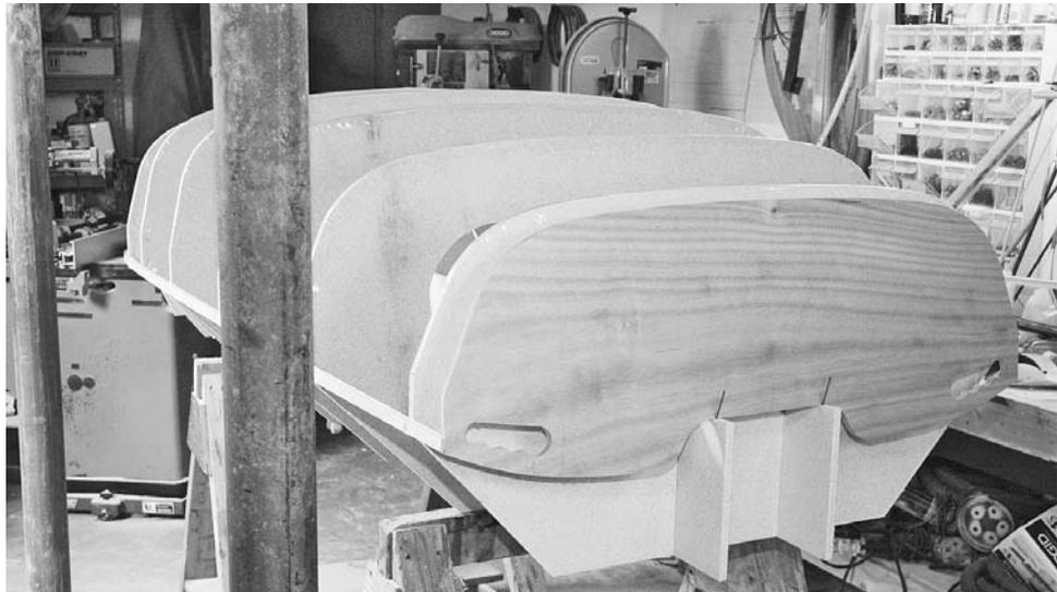
**Figure 11-10.** The Coot has transoms (flat ends) at both ends. The transoms have been pre-coated with epoxy to protect them from glue drips and other abuse. This strongback has supports to hold the transoms in the correct position.
