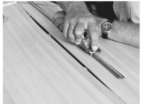
**Figure 6-40.** Start tapering the strip at one end. Here a piece of scrap protects the boat while allowing me to work right where I need the strip. Test the fit at this end, planing farther along as the tip starts to fit well. Try not to go beyond the previously made marks as this will indicate you are losing some of your margin of error for fitting the other end.
