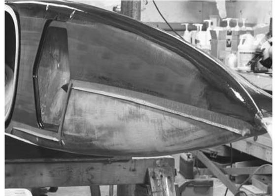
**Figure 13-71.** Low-viscosity epoxy runs off the boat quickly. This makes it hard to get a full fill coat on the sides. Here I have turned the boat on edge to help get the sides of the kayak filled up. Note that the bottom edge of the tape has been bent up to act as a drip edge, keeping drips from just running straight across the tape.
