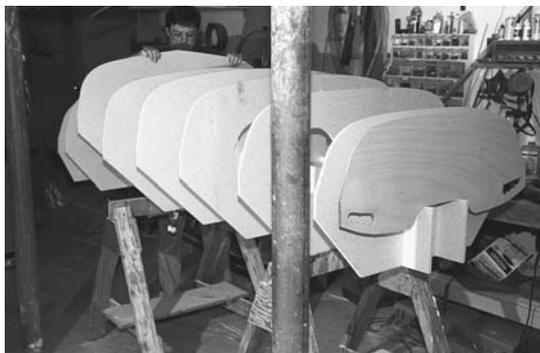
**Figure 5-18.** *The slotted strongback is very simple to set up. Two long beams with slots cut in them accept matching slots on the forms. Drop the forms into the slots, make sure they are seated all the way down, and you are good to go.*
