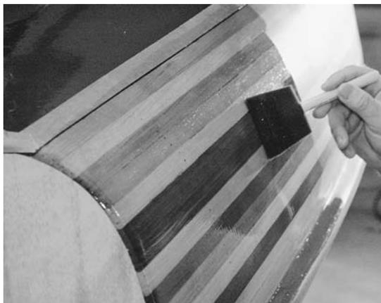
**Figure 10-12.** Finally, lightly tip off bubbles with quick, even strokes. Brush in one direction, from the drier side to the wetter. Lift up the brush while you are moving. Double-check for holidays as you work. As soon as you finish one section, move on to the next section. This is not a time to answer the phone or go eat cookies. Do the whole boat without stopping. When you are done, peel off the tape and leave the area so you don't stir up dust.
