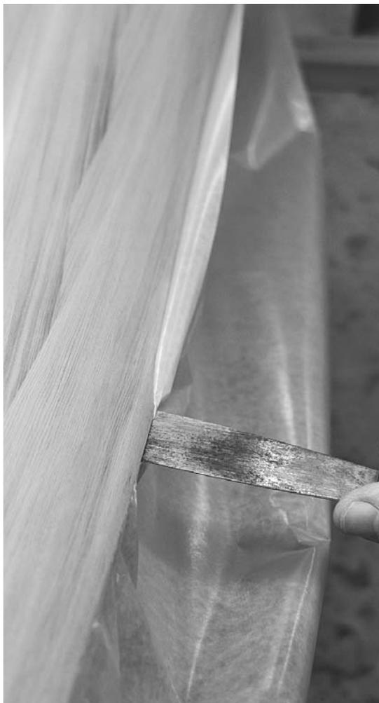
**Figure 13-43.** Slide a sheet of waxed paper in between the deck and hull to protect the other half as you stain and epoxy. The seam may be quite tight—I find that a putty knife helps coax the paper into the sheer seam.
