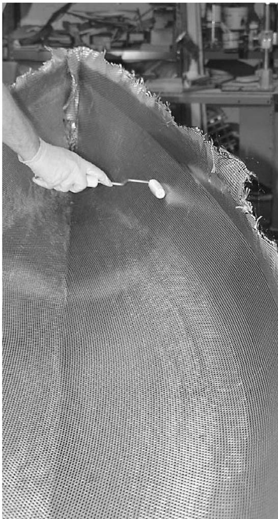
**Figure 12-26.** A bubble roller (a grooved roller tool intended for removing bubbles from fiberglass) helps press down the cloth tight against the wood, driving any excess resin under the cloth up to the surface. While not really useful with light fiberglass, the roller can help create a lighter layup with this thicker hybrid cloth.
