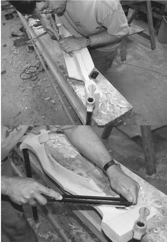
**Figure 12-34.** I cut the backrest from 2-inch-thick Sitka spruce. The top and bottom pieces were cut as nested pieces from the same piece of wood on a band saw with the table set at an angle. The glued up pieces were shaped with rasps and microplanes.
