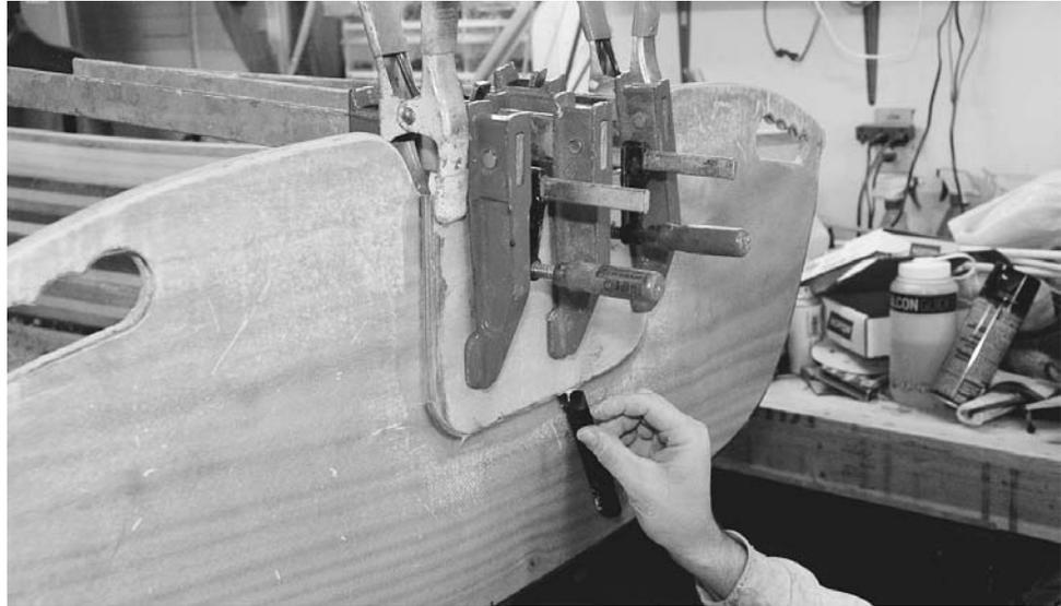
**Figure 11-36.** If you want to use a motor on your boat, you need to reinforce the stern. Set a piece of fiberglass-covered plywood in epoxy thickened with colloidal silica and clamp it onto the back. Clean up any squeezed-out glue, leaving a little fillet between the transom and the edge of the reinforcement.
