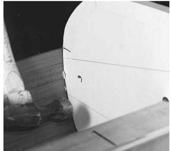
**Figure 6-18.** If you have not applied too much hot-melt glue during your staple-free construction, you should be able to break the glue free with a sharp rap of a hammer. The forms need to be released from the strongback enough that they can move without breaking.
