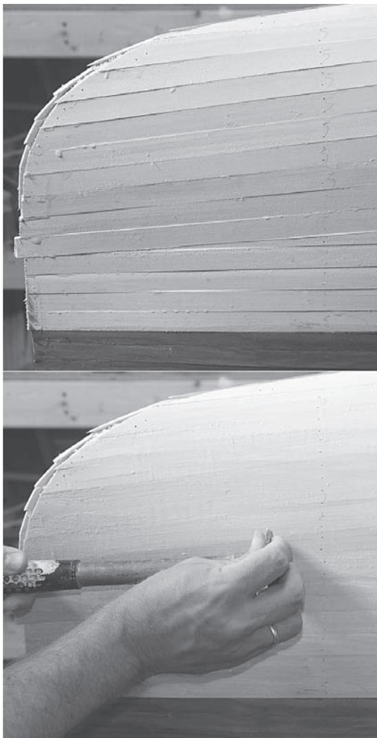
**Figure 7-1.** Although the scraper is really good at removing glue drips, it can also do a lot of fairing pretty quickly. The scraper needs to be held firmly so it does not chatter and skip.
