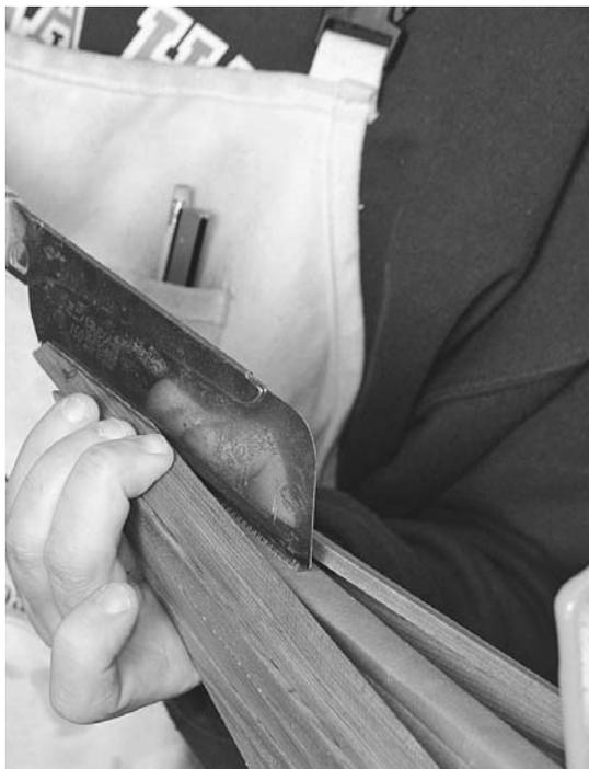
**Figure 13-29.** You start the deck much like the hull. This time match your rolling bevel to the bevel on the top strip of the hull. The ends of this design meet in a V-shape that requires a matching taper on the strips approaching from both sides. Rough this out with a plane and then fine-tune it by dragging a saw through the seam.
