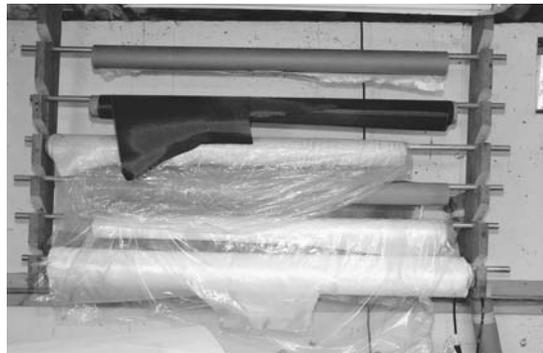
**Figure 2-4.** To help keep the fabric clean and undistorted, make a fabric dispensing rack from 2 by 6 lumber and electrical conduit to hold the rolls. Shown on this rack are black carbon fiber cloth, Kevlar (straw colored), and some different kinds of fiberglass. The plastic keeps dust off the material.
