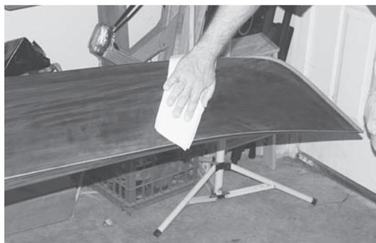
**Figure 10-8.** Remove dust from the surface of the boat before varnishing by vacuuming, rinsing it with water, and then wiping with a tack cloth.
