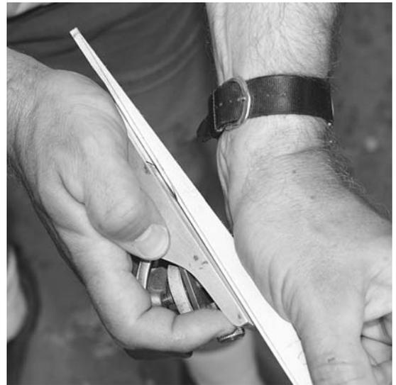
**Figure 6-23.** Tapers can be planed into the ends of strips using a push or pull stroke. With a sharp plane you may be able to accurately shape some long tapers without support, but as they get longer you may want to back up the strip with another scrap piece.
