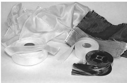
**Figure 2-5.** Reinforcing fabrics are available in a variety of materials. The white fabrics on the left are fiberglass, which becomes clear when saturated with resin. The black carbon fiber (top right) stays black. Woven tapes of different widths (middle right) are available for reinforcing and joining parts. The spool on the lower right contains carbon fiber “tow,” an unwoven roll of fibers that can be used to make reinforcing ribs.
