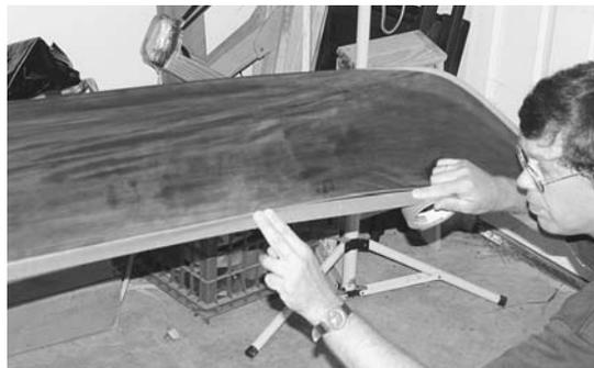
**Figure 10-7.** Mask off the lower edge of any area to be varnished to control any drips that may accumulate. Fold up the bottom edge of the tape to create a drip edge. Varnish the hull about 1 foot at a time, switching sides every 2 feet so you maintain a wet edge along the centerline. Remove the tape a minute or so after you have finished varnishing. Let the varnish dry, and then flip the boat over and repeat for the deck.
