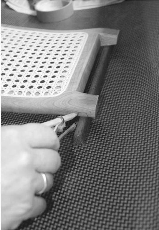
**Figure 12-38.** With the seat stringer on the bottom of the boat, I wanted to get the seat as low as possible. I notched the cross arms to fit over the stringer, which let it nestle down on the bottom. For a higher-mounted seat, this would not be necessary.
