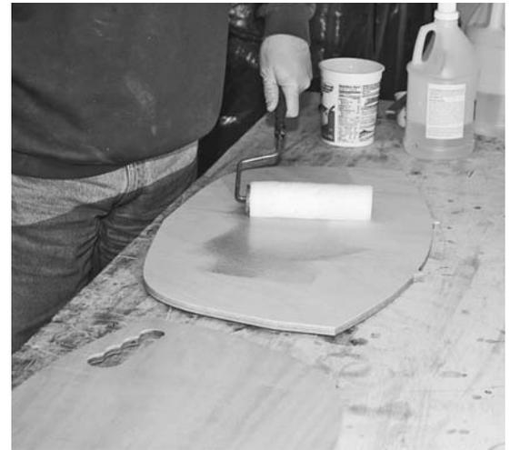
**Figure 5-31.** Any plywood parts such as transoms that will remain in the boat after stripping should be coated with epoxy to protect the wood from glue drips and other damage.
