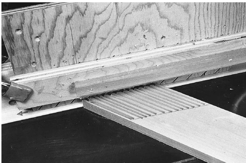
**Figures 5-11 and 5-12.** The coves and beads are milled on the strips on a router table. Set the router up so the bit is turning opposite of the feed direction of the strip. When the bit height has been adjusted so it cuts down the middle of the strip and the fence has been adjusted so the depth is just deep enough, install feather boards. One board should hold the strip down on the table, with another pressing it against the fence.
