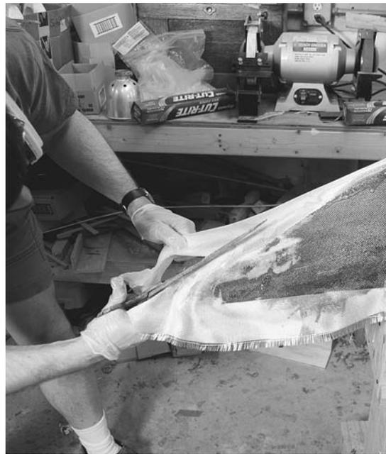
**Figure 9-17.** Most wrinkles need to be moved toward the ends of the boat. Depending on the shape of stem, you may need to trim the glass at the ends. While it is possible to wrap the trimmed glass around either side, I find it easier to let it come off straight and then trim it off later.
