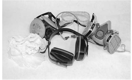
**Figure 3-15.** Although many of the materials used in strip building may seem benign, there are risks. You should strongly consider wearing hearing and eye protection whenever you run power tools. Wood sawdust is considered carcinogenic; a good dust mask (upper left) will keep it out of your lungs. Even though epoxy does not smell much, an organic vapor respirator (upper right) is highly recommended. You also don't want to get epoxy on your skin, so wear gloves.
