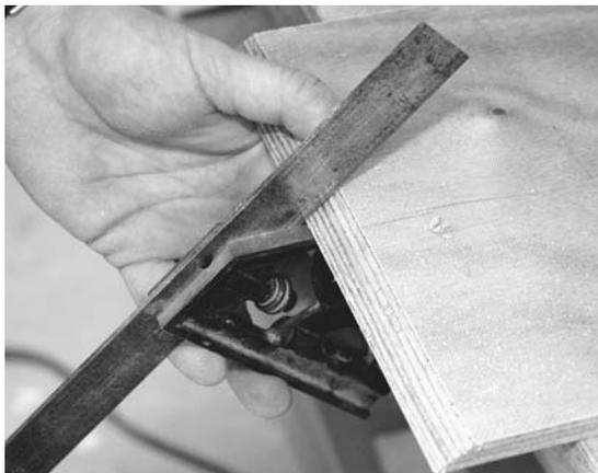
**Figure 11-30.** The ends of the middle-seat supports need to have 45-degree-angle mitered bevels on the inside edges to create a tight joint. Plane this with a block plane and check it with a combination square. Don't plane this down to a knife-sharp edge because you may end up changing the length of the part. Instead, watch the layers of plywood as you plane down through them and stop when you hit the bottom layer.
