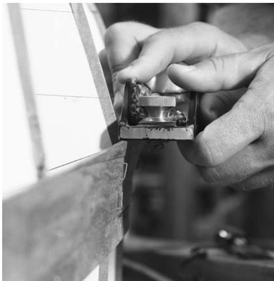
**Figure 12-16.** Clean up the edge with a rabbet plane. Try for a smooth, fair curve with a consistent angle on the bevel.
