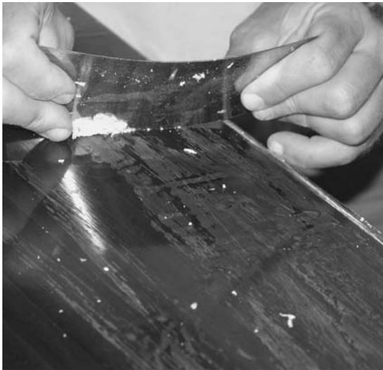
**Figure 10-2.** A cabinet scraper does a good job of leveling small irregularities. It can be used with a lot of precision to knock down a small drip. Larger drips can be attacked with a rasp or paint scraper.
