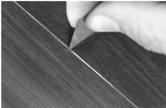
**Figure 13-45.** It is very hard to create a crisp edge with stain because it soaks under masking tape very easily. You can stain right over any transition, then scrape off the stain. Here I stained the whole boat and then scraped the stain off the maple feature line with a modified utility knife blade.
