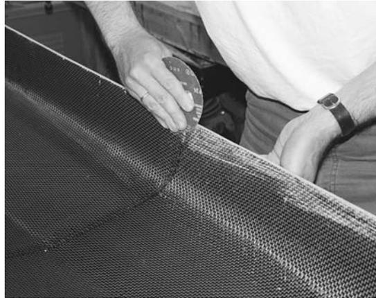
**Figure 9-31.** *Before joining the deck and hull, rough up the epoxy and fabric along the edge to assure a strong bond.*
