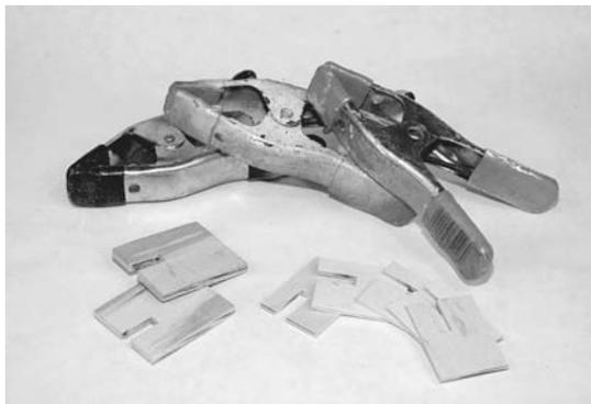
**Figure 3-11.** To temporarily hold the strips in place, you can clamp little U-shaped jigs that fit over the strips to the forms.
