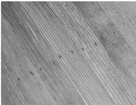
**Figure 6-14.** On my own boats, I happily pump the strips full of staples. I feel they are an honest side effect of building a boat, and from a distance you just won't see them. A wooden boat will suck up all the perfectionism you can feed it, and you need to pick your battles. Staple holes should not be considered a flaw, but instead an indication of the fact that the boat is made by hand.
