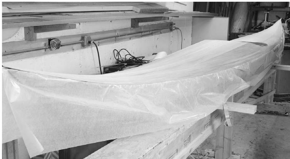
**Figure 7-17.** With a decked boat you could remove the hull or deck while sanding, staining, or glassing the other half, but often the safest place for it is on the forms. Inserting waxed paper at the sheeline will protect the bottom half as you work on the top.
