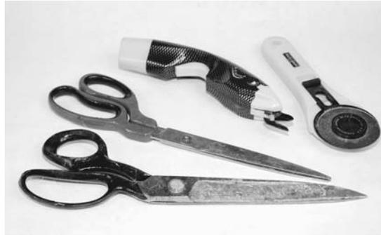
**Figure 3-9.** Fiberglass is usually cut with scissors. They will likely get coated with epoxy, and cutting glass dulls them, so don't go to the sewing kit thinking no one will notice. Second from the right is a battery-powered fabric cutter that may be worth the investment if you do a lot of fiberglass work. If you have a smooth surface to cut on, the rolling cutter on the right works well for cutting strips of cloth.
